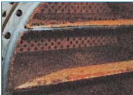
**Corrosion, in general, and pitting corrosion, in particular, must be guarded against in order to ensure the long-term integrity of the cooling system.**
