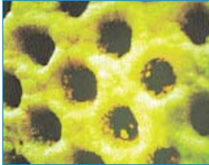
**Scale thickens the barrier to heat transfer, thus reducing the efficiency of the cooling system.**
